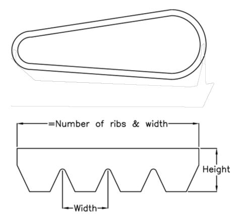
$\begin{array}{ll} \text{Datum Llength} = 1321 \\ \text{Height} &= 3.5 \\ \text{Number of ribs} = 15 \\ \text{Pitch} &= 2.34 \end{array}$
